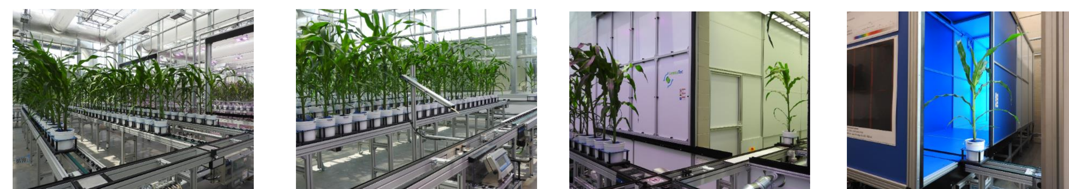
Figure 4: LemnaTec Scanalyzer 3D Plant Phenotyping System
