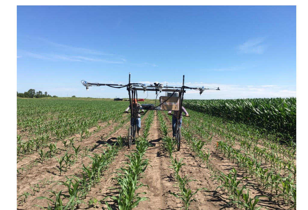
Fig 4. Image-based phenotypes collection for hybrids in early stage using phenotyping platform developed by the Ge lab.
